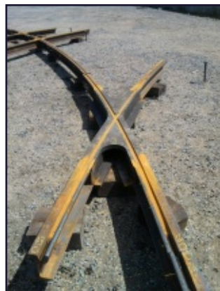
A special sandwich frog with the functional part of wear-resistant sheet metal HARDOX® 450.
