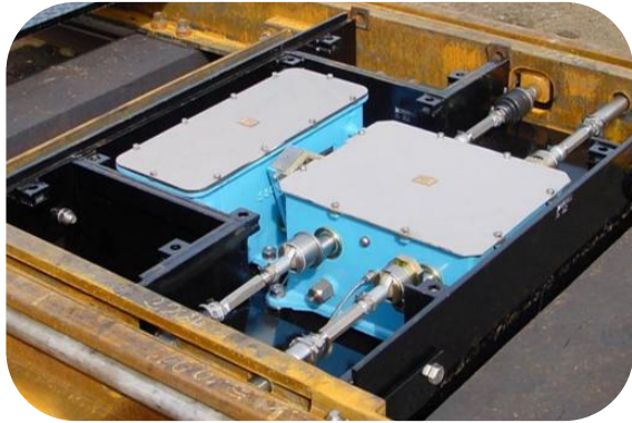
automatic point system VSP-1-K
